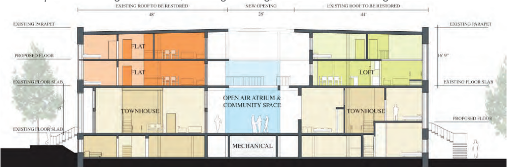
Section Reveals the Stacking of Units and Innovative Reuse of Existing Floor Slabs
